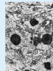
DC (High-strength/toughness type) ×100
