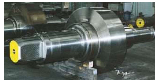
Universal horizontal roll (after building-up)
